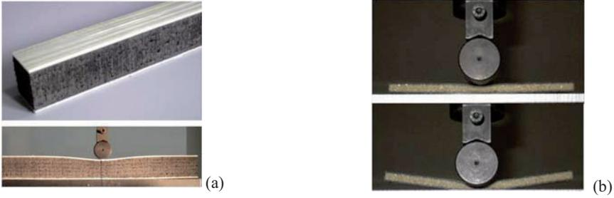
Fig. 3. Sample S1 (a) and S3 (b) during the indentation test (cylindrical indenter diameter 25 mm).
