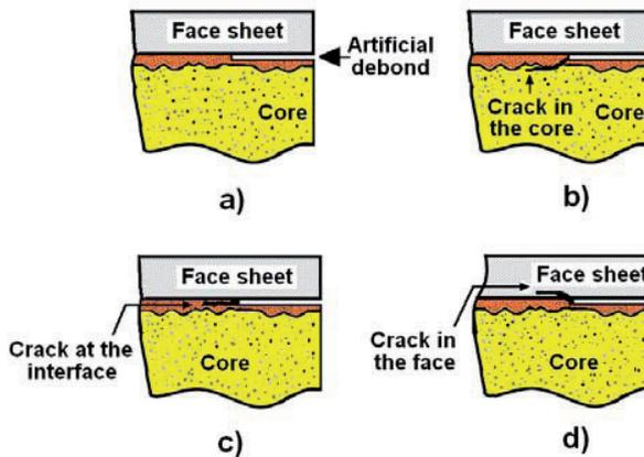
**Fig. 2.** Schematic initial crack locations a) artificial debond, b) debond crack in the core just below the face/core interface, c) debond crack directly in the face/core interface, and d) debond crack in the face laminate.
