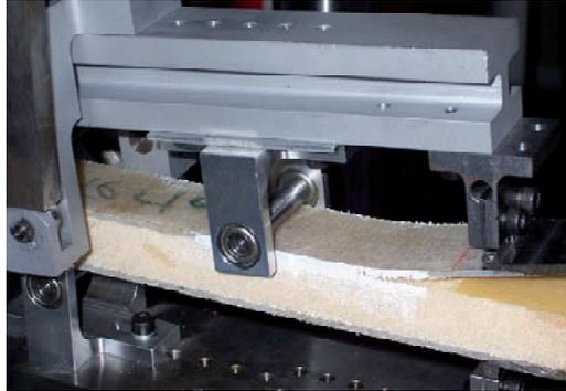
**Fig. 4.** Observed crack propagation path in a MMB specimen during testing, with crack growth in the core.
