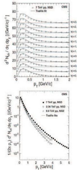
**Fig. 13.** Transverse momenta distributions of charged hadrons in pp collisions, as measured by the CMS Collaboration at LHC, corresponding to 0.9, 2.36 and 7 TeV. At these energies it has been obtained  $(q, T) = (1.13, 0.13 \text{ GeV})$ ,  $(1.15, 0.14 \text{ GeV})$ ,  $(1.15, 0.145 \text{ GeV})$  respectively. See details in [64,65].
