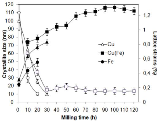
**Fig. 3.** Dependence of the microstructure parameters of the metallic phases on the milling time: the calculated crystallites sizes (Empty markers) and the calculated lattice strains (Full markers).
