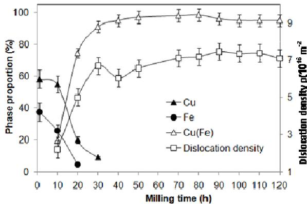
**Fig. 4.** Evolution of the phase proportions of the identified phases and the dislocations density as a function of milling time.
