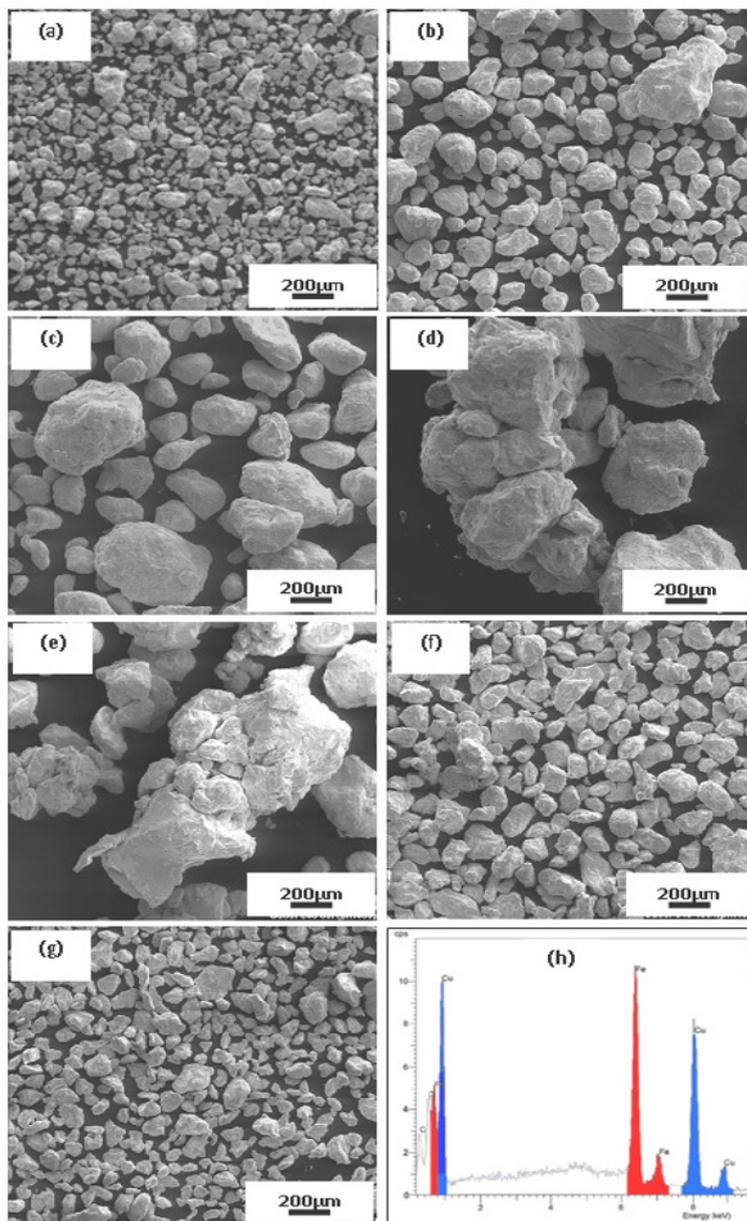
**Fig. 1.** Typical scanning electron micrographs (secondary electron image mode) corresponding to mechanically milled Cu-Fe powders (initial composition 60% Cu): (a) 1h, (b) 20h, (c) 40h, (d) 60h, (e) 80h, (f) 100h, (g) 120h and (h). The EDX corresponds to 100h.
