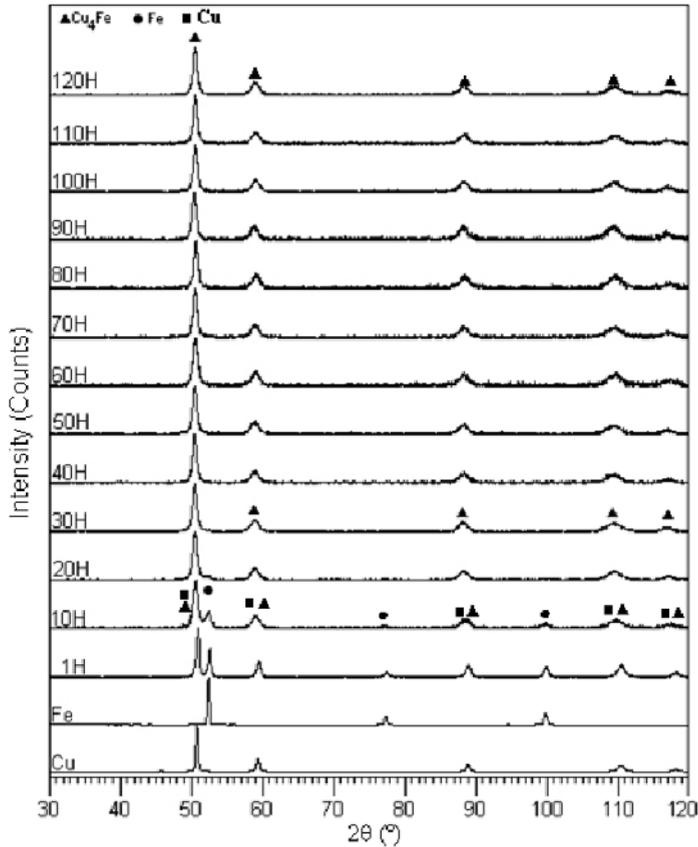
**Fig. 2.** XRD patterns of X-ray diffraction pattern of the MA Cu-Fe powders as a function of milling times.
