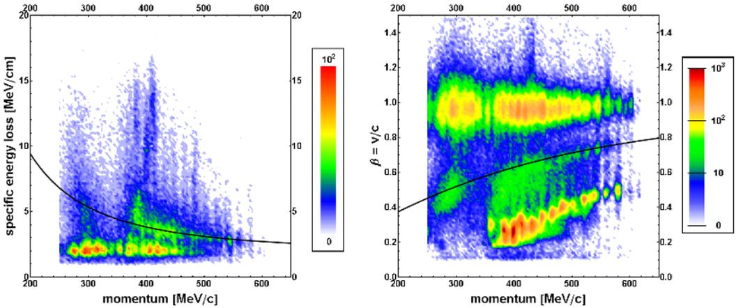
**Figure 1.** Identification of positively charged particles by their specific energy-loss (left) and their relative velocity (right) in the momentum range of the KAOS spectrometer. The expectation for kaons is indicated by the solid lines. Pre-selection cuts have been applied to suppress the background of positrons and pions (found at  $dE/dx \approx 2\text{--}3$  MeV/cm and  $\beta \approx 1$ ), and of protons (found at  $\beta \approx 0.2\text{--}0.4$ ).
