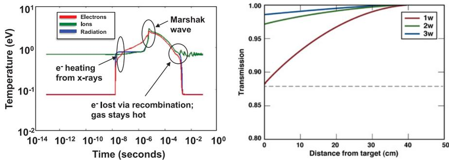
Figure 2. Laser beam propagation through 6  $\mu\text{g}/\text{cc}$  xenon results in minimal losses.
