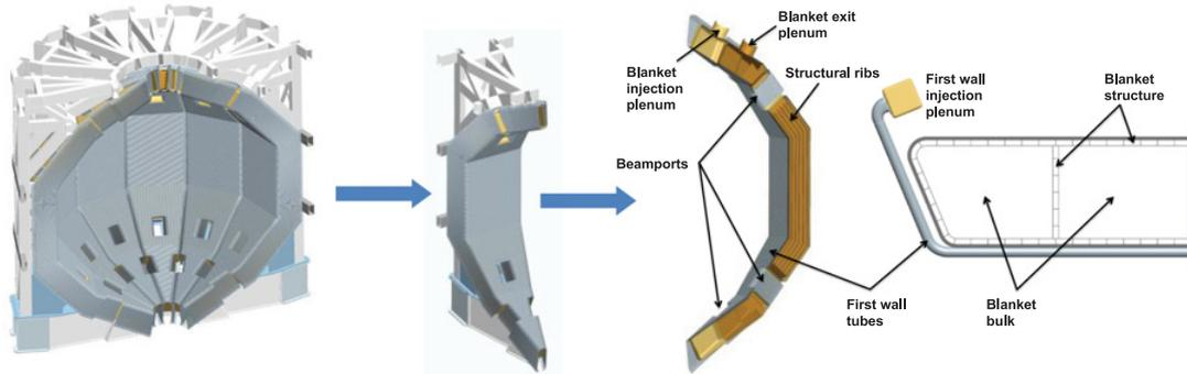
Figure 3. LIFE chamber design is modular, replaceable and fabricated from existing materials.
