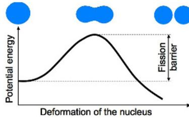
**Figure 1.** Schematic plot of the potential energy surface of the nucleus as a function of deformation, which shows the fission barrier and the associated shapes of the nucleus.
