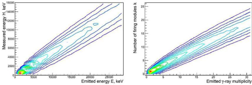
**Figure 3.** Measured energy response (left panel) and fold response (right panel) of GAMMASPHERE to the emission of a series of 898 keV gamma rays (see references [16–18] for details on the calibration method).
