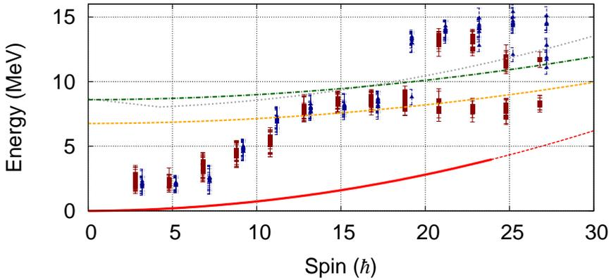
**Figure 5.** Saddle point energies extracted from the entry distributions measured at 219 MeV (red squares) and 223 MeV (blue triangles). Multiple unfolding results lead to multiple points per spin value. The black full line is the yrast energy, the dotted grey line represents the neutron separation energy. See text for more details.
