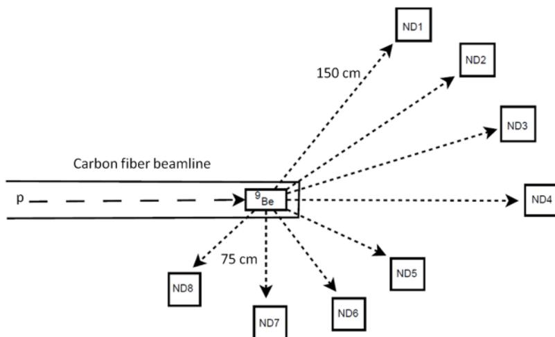
**Figure 1.** Schematic view of the experimental setup. The Beryllium target, installed inside the carbon fibre tube, is connected to a digital beam current integrator. The near/small detectors are placed at 75 cm from the Be target while the far/large detectors at 150 cm. Both small and large detectors were moved to cover 16 angles from 0° to 150°.
