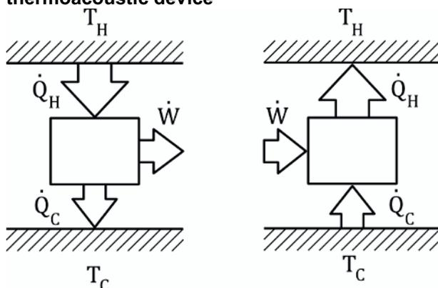
**Figure 1.** Schematic of function of thermoacoustic engine (left) and thermoacoustic heat pump (right)
