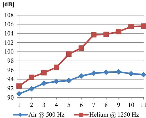
Average value of intensity of sound was determined for device with air as working gas roughly 94 dB and for device with helium as working gas roughly 100 dB.
