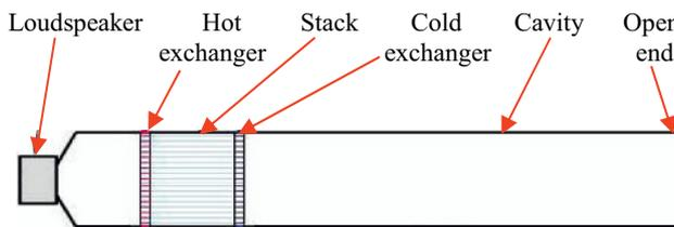
**Figure 3.** Schematic of thermoacoustic heat pump
