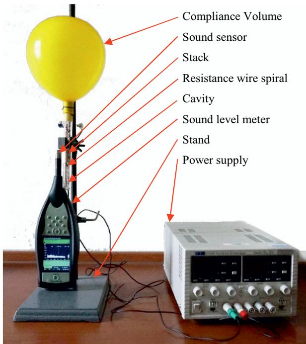
Figure 1. Scheme of thermoacoustic device
