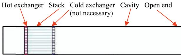
**Figure 2.** Schematic of thermoacoustic engine
