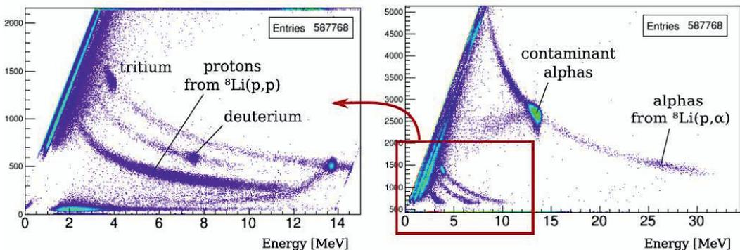
**Figure 4.** Bidimensional energy spectra obtained using a Si telescope at  $\Theta_{lab}=10^\circ$ , in the large chamber after the second solenoid, with the secondary beams focused on a  $[\text{CH}_2]_n$  target. The spectrum on the left is a zoom of the spectrum on the right.
