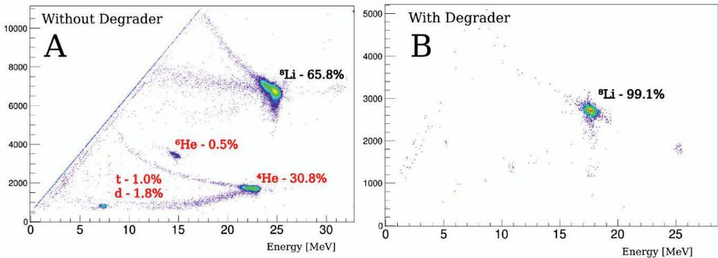
**Figure 3.** Bidimensional energy spectra obtained using a Si telescope at  $\Theta_{lab}=10^\circ$ , in the large chamber after the second solenoid, with the secondary beams focused on a gold target. Spectrum A was obtained without a degrader and spectrum B with a degrader.
