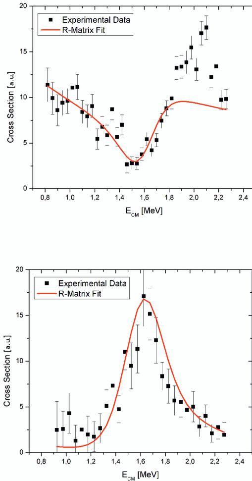
**Figure 5.** The excitation function of the  ${}^8\text{Li}(p,p){}^8\text{Li}$  reaction, together with a fit by the R-matrix calculation is shown on the top. On the bottom is the excitation function of the  ${}^8\text{Li}(p,\alpha){}^5\text{He}$  reaction, together with a fit by the R-matrix calculation.
