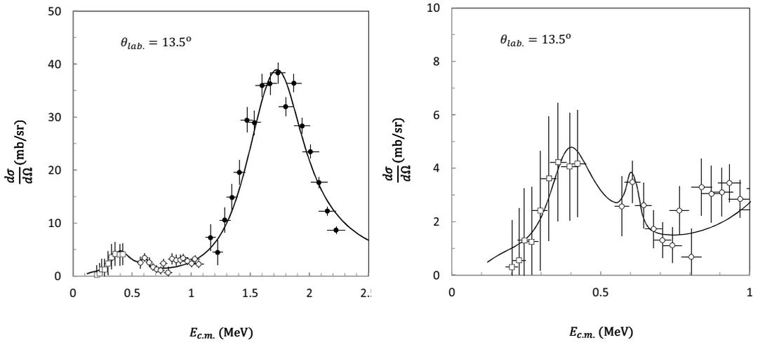
**Figure 1.** The spectrum on the left shows the  ${}^8\text{Li}(p,\alpha){}^5\text{He}$  differential cross sections at  $\theta_{\text{lab}} = 13.5^\circ$ , with the  $R$ -matrix fit (solid line.) In the spectrum on the right we present the same reaction, performing a zoom on the low energy resonances and their  $R$ -matrix-fit.
