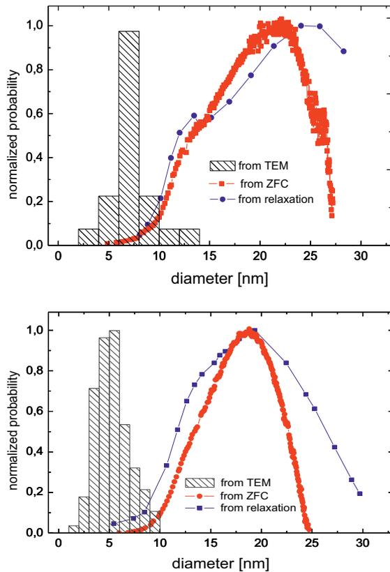
**Fig. 6.** Particle size distributions obtained geometrically from TEM pictures, and magnetically from ZFC-curves, as well as from magnetic relaxation data for uncoated FeNiB (upper panel) and coated FeNiB/SiO<sub>2</sub> (lower panel).
