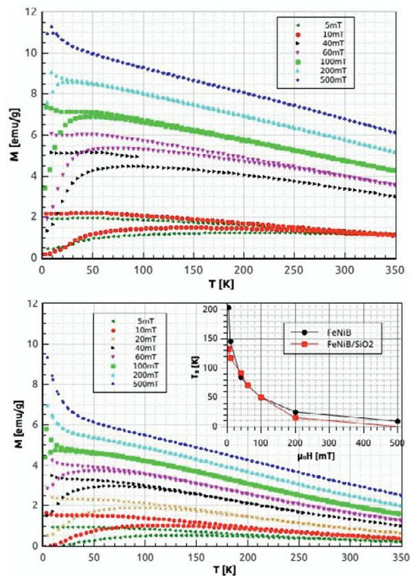
**Fig. 2.** Temperature dependence of magnetization of FeNiB (upper picture) and FeNiB/SiO<sub>2</sub> (lower picture) obtained by zero-field-cooled (lower curves) and field-cooled (upper curves) measurements. **Inset:** field dependence of blocking temperature  $T_B$  for both samples.
