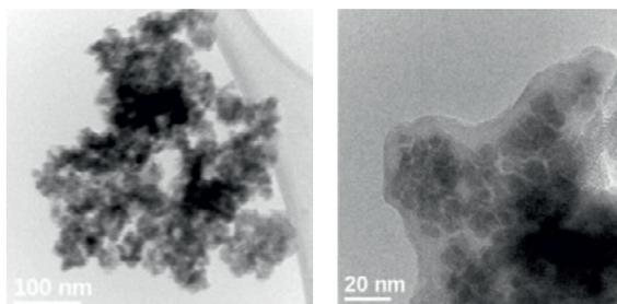
**Fig. 1.** TEM pictures of FeNiB (left) and FeNiB/SiO<sub>2</sub> (right).
