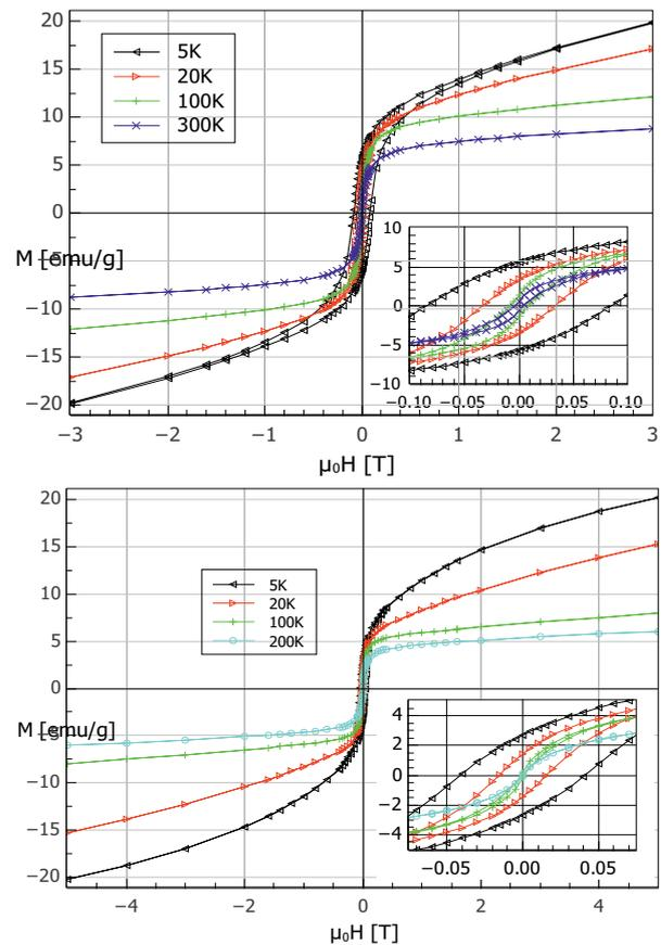
**Fig. 3.** Field dependence of magnetization of FeNiB (upper picture) and FeNiB/SiO<sub>2</sub> (lower picture) for selected temperatures. **Insets:** Enlargement of inner part of hysteresis loops.
