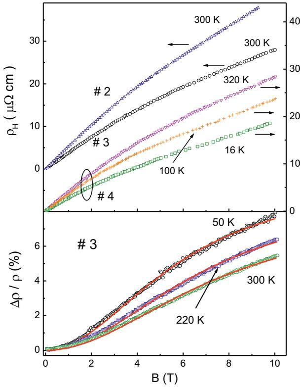
**Fig. 1.** The magnetic field dependences of  $\rho_H$  (top panel) and of  $\Delta\rho/\rho$  (bottom panel). The lines are calculated as described in the text.
