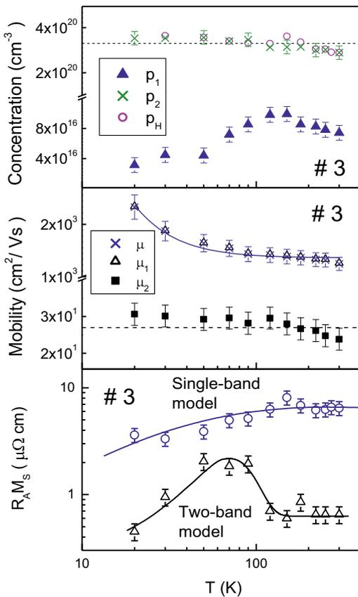
**Fig. 3.** Temperature dependences of  $p_1$ ,  $p_2$  and  $p_H$  (top panel), of  $\mu_1$ ,  $\mu_2$  and  $\mu$  (middle panel) and of  $R_A M_S$  (bottom panel) in # 3. The lines are to guide the eye.
