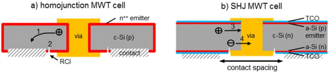
**Figure 1.** Loss mechanisms in MWT cells: In homojunction MWT cells (a) the lateral current towards the base contacts (1) and losses at the RCI (2) are critical. In SHJ-MWT cells (b) additional loss mechanisms are caused by via surface recombination (3) and via-base leakage (4).
