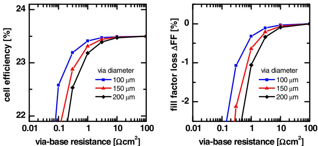
**Figure 5.** Simulated solar cell efficiencies and FF for different via-base resistances and different via diameters. Below  $1 \Omega \text{cm}^2$ , the cell performance drastically decreases.
