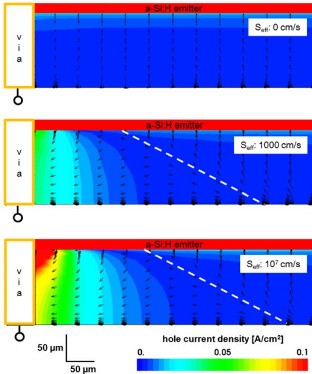
**Figure 7.** Hole current densities and vectors for different via surface recombination velocities for a  $100\ \mu\text{m}$  via at the operation point of the cell. The vectors point in the direction of the conventional current flow.
