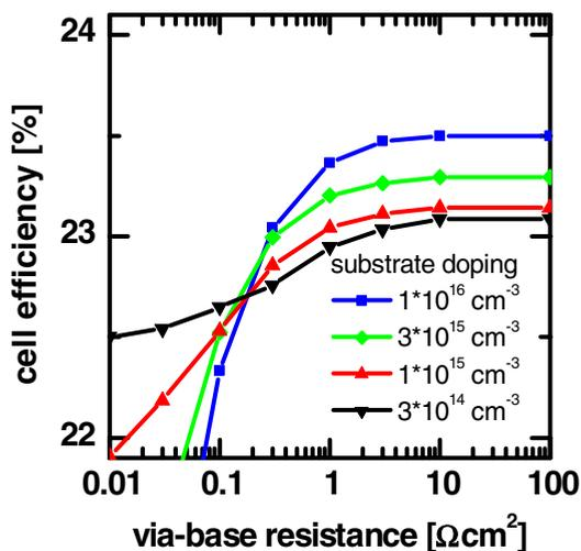
**Figure 6.** Simulated solar cell efficiencies for different via-base resistances and different substrate doping levels. The influence of the via-base leakage decreased for lower substrate doping.
