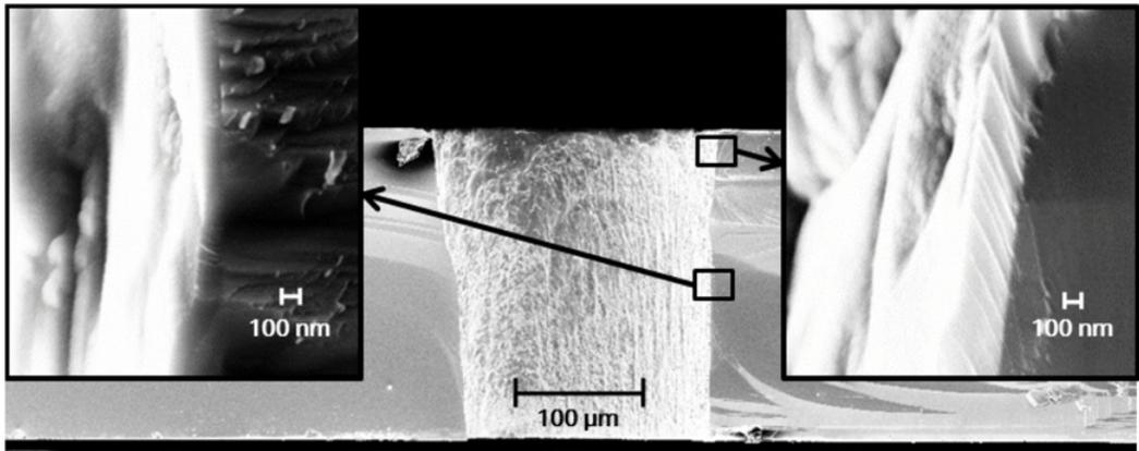
**Figure 3.** SEM cross-section through a via after deposition of 550 nm a-Si:H in a PECVD process. The a-Si:H thickness is 300 nm at via top (right) and below 100 nm at the via mid-position (left), respectively.
