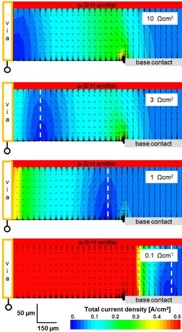
**Figure 4.** Current densities and vectors for different via-base contact resistances for a  $100\ \mu\text{m}$  via at the operation point of the cell (simulated area as indicated in Fig. 2). The vectors point in the direction of the conventional current flow.
