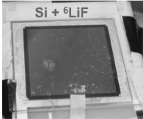
**Figure 2.** The silicon detector sandwiched between two  ${}^6\text{LiF}$  neutron converters.
