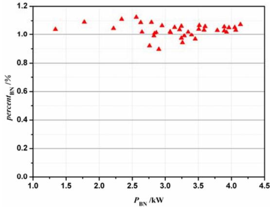
**Figure 10.** Percentage of the power absorbed by BN window. As shown in the Fig.10, the percent of power absorbed by BN is 1.05%. The windows of Gyrotron and near the EC launcher are CAD in 140GHz. But the 140GHz systems have not been injected into plasma.
