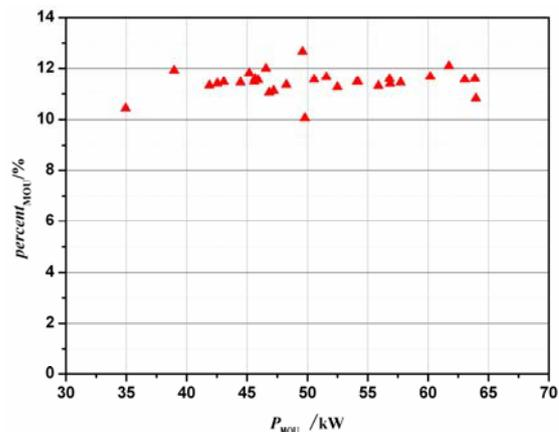
Figure 8. The percentage of the spurious mode power absorbed by MOU in 68GHz system.
