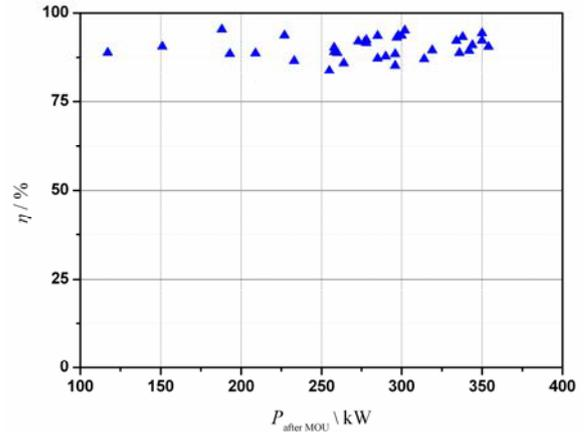
**Figure 12.** Transmission efficiency of transmission line in 68GHz system
