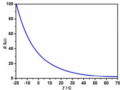
Figure 3. The typical curves of NTC
