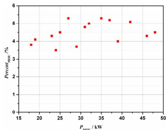
Figure 9. The percentage of the spurious mode power absorbed by MOU in 140GHz system.
