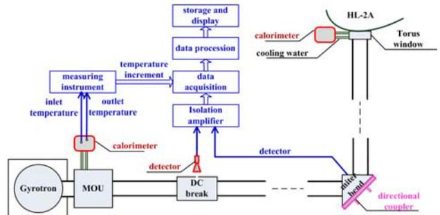
Figure 4. The location schematic diagram of calorimeters installed
