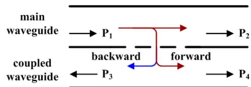
**Figure 13.** Schematic diagram of a coupler
