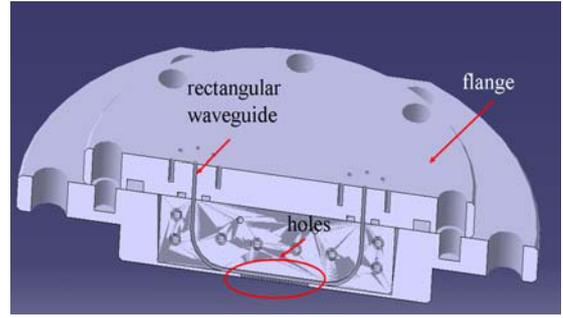
**Figure 14.** Structure of the directional coupler
