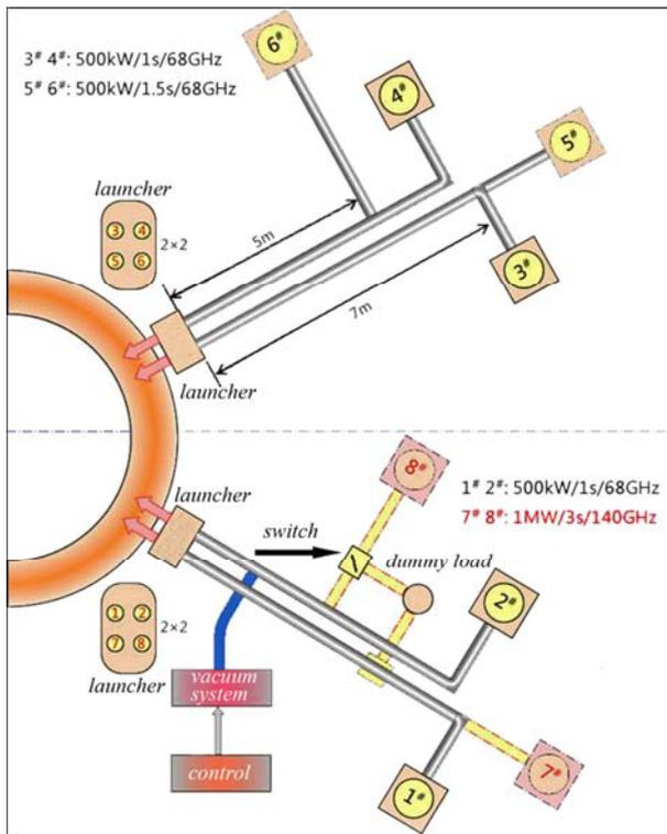
**Figure 11.** Schematic of ECRH system
