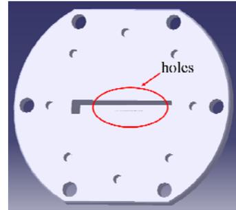
**Figure 15.** Structure of coupled holes on reflect mirror
