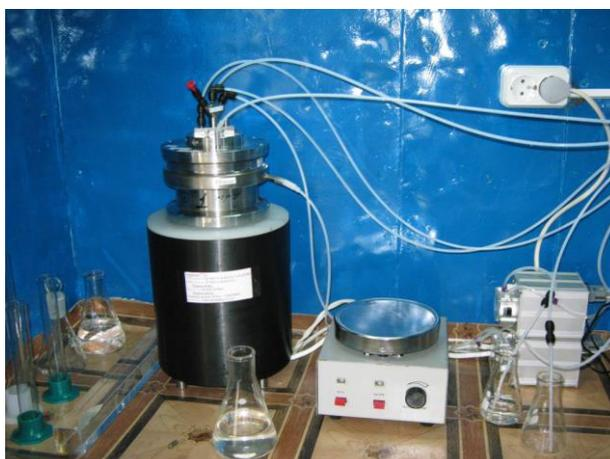
**Figure 7.** The main part of the centrifuge extractor complex.
