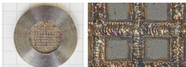
**Figure 11.** The target disc with pressed Mo powder after processing by laser beam (left), zoomed (right).
