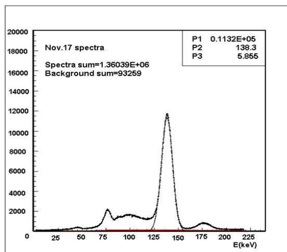
**Figure 6.** The energy spectrum from the irradiation of the  $\text{MoO}_3$  measured with a NaI(Tl) detector.
