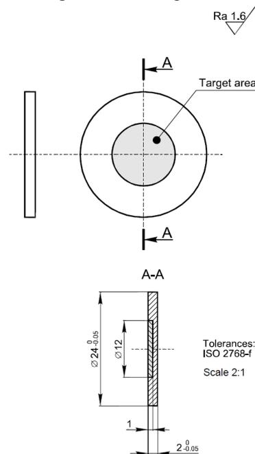
**Figure 9.** Solid target disc.
