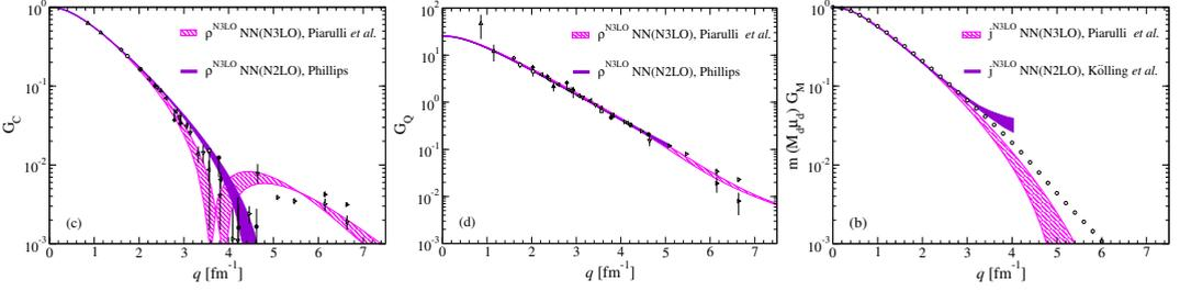
**Figure 3.** **Left:** Deuteron charge form factor from Ref. [31] (magenta hatched band) and Ref. [36] (purple solid bands) compared with experimental data (black points). **Middle:** Same as left panel but for deuteron quadrupole form factor. **Right:** Deuteron magnetic form factor from Ref. [31] (magenta hatched band) and Ref. [37] (purple solid band) compared with experimental data (open circles).
