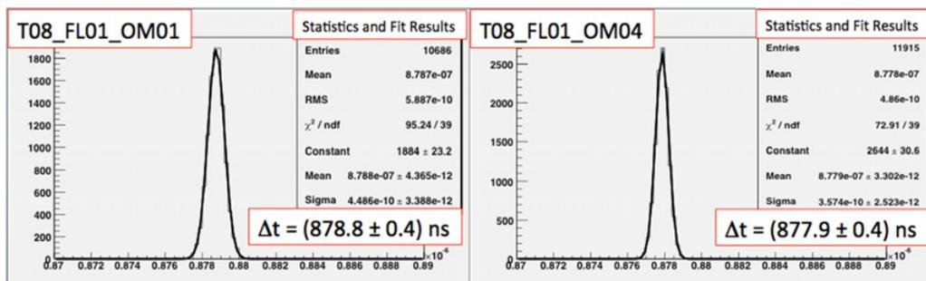
**Figure 1.** Distribution of the time differences (in seconds) between CH2 of the TDC (the MPPC digital output) and CH1 (the reference signal). Both the measurements have been done setting the same value for the number of readings acquired with the TDC, and the statistics is comparable for the 2 OMs. The result of a Gaussian fit is superimposed, showing comparable uncertainties (400 ps) for the two set of measurements.
