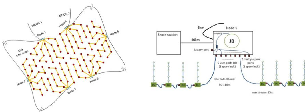
**Figure 2.** The MEUST generic submarine topology (left) and the layout of the 4-DU chain connected on the node (right).
