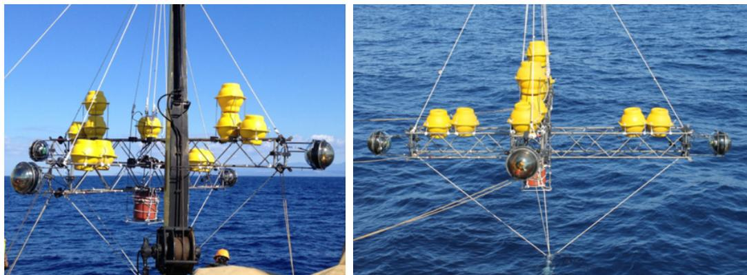
**Figure 3.** Left: A floor lifted from the deck of R/V AEGAEO. Right: A floor just before submersion.
