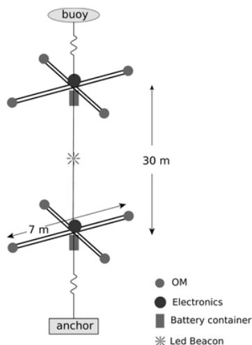
**Figure 1.** A schematic representation of the GRBNeT prototype detector.
