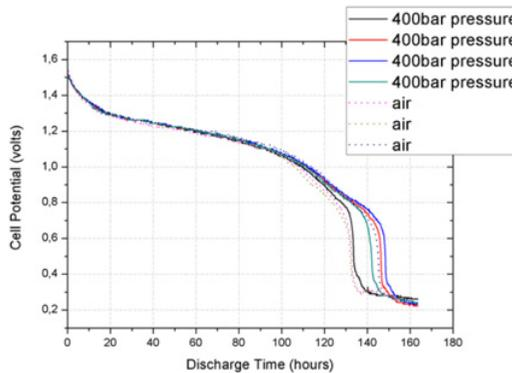
**Figure 2.** The voltage ( $V$ ) of seven batteries versus the discharge time of each cell. Dotted/solid lines correspond to batteries discharging in air/under pressure of 400 bar respectively.
