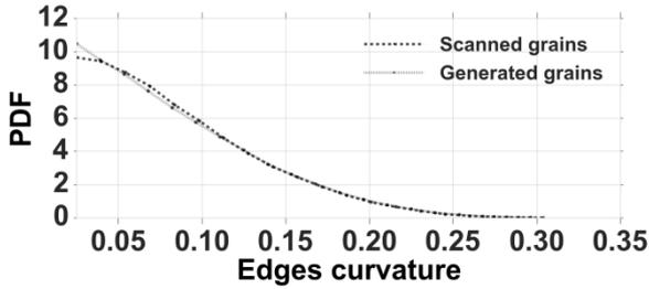
**Fig.6.** Edge curvature (Curvature = variation of normal directions; faces=low curvature, edges=High curvature) (PDF)
