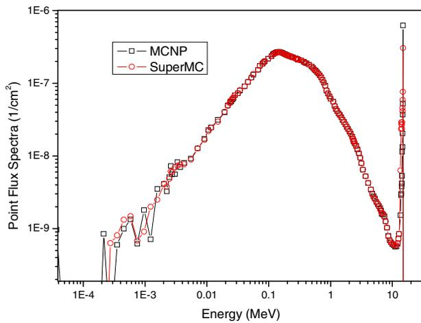
**Fig. 3. Comparison of point neutron flux of Th sphere experiments with 14MeV neutron source**
