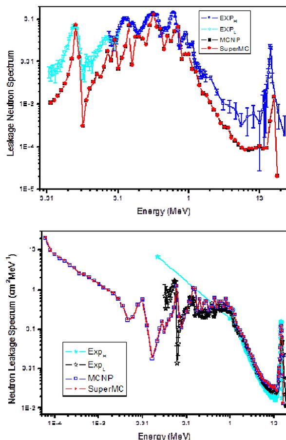
Fig.1 Comparison of neutron leakage currents of Osaka benchmark experiments (Up: Iron, Down: Nickel)
