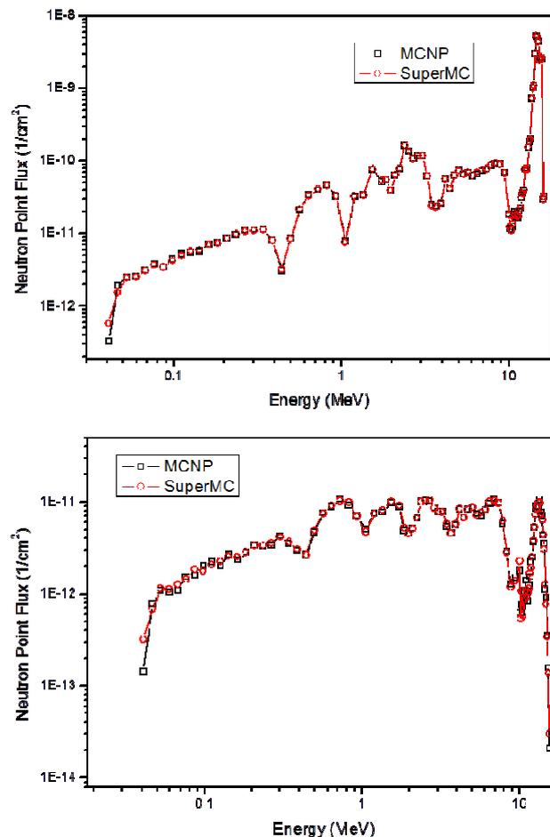
Fig. 2. Comparison of point neutron flux of FNS oxygen slab benchmark experiments (Up: 0 degree, Down: 66.8 degree)
