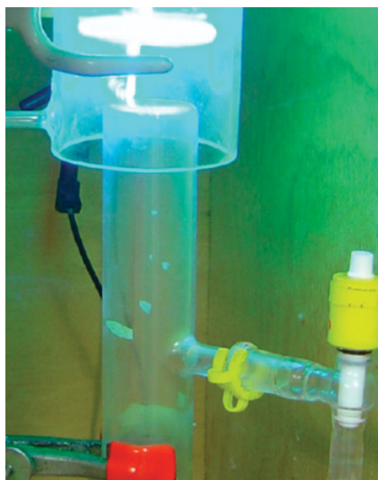
Figure 1. Closed cell equipped with a Suprasil window and a stopcock.
