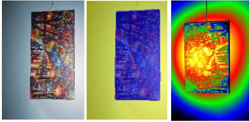
Figure 2. (Left) Picture taken by the microprocessor - (Middle) Segmentation map - (Right) Final illuminance measured with a luminance camera.
