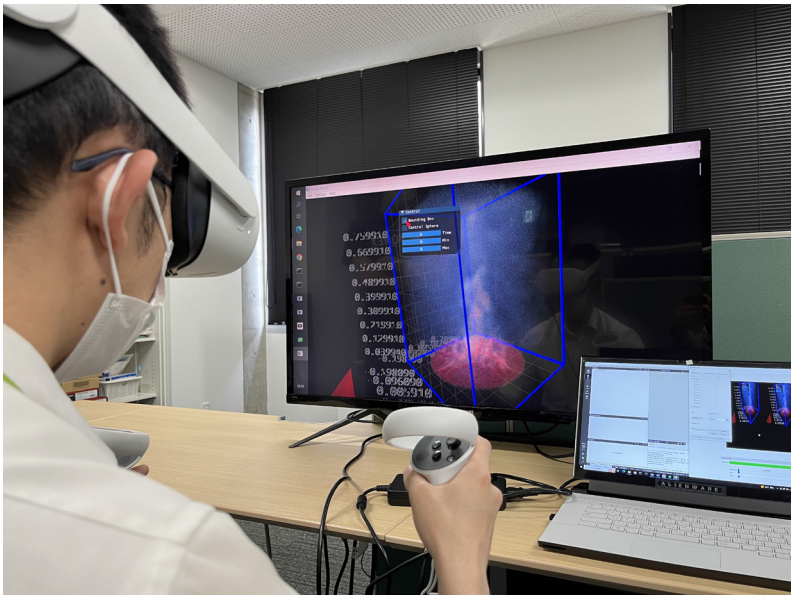
Figure 4. Debris air cooling analysis using VR IS-PBVR with HMD Meta Quest Pro.
