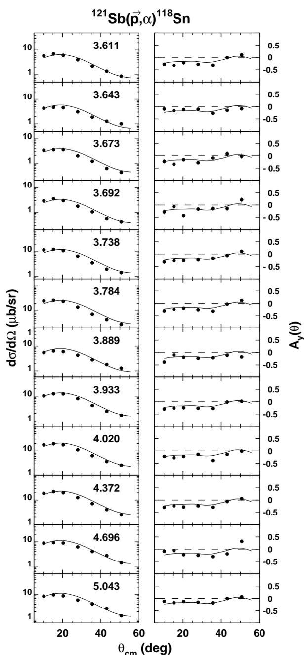
**Fig. 4.** Angular distributions of cross sections and asymmetries for some of the 23 positive parity daughter states of  $^{118}\text{Sn}$  homologous to the G.S.  $9/2^+$   $^{117}\text{In}$  parent state. Dots refer to the experimental values of the daughter states and solid lines to the experimental values of the parent state.
