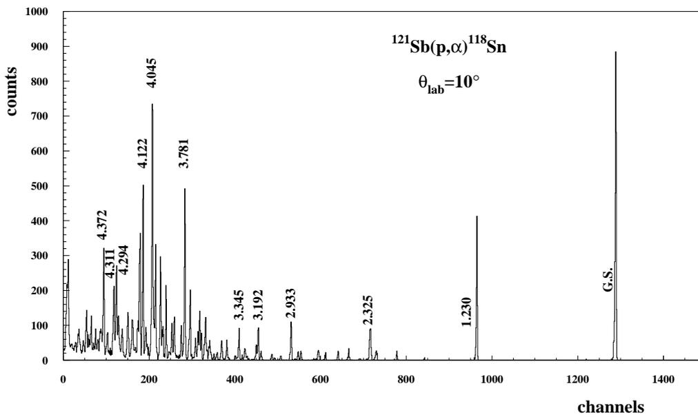
Fig. 2. Energy spectrum of  $\alpha$  particles measured at  $10^\circ$  for the  $^{121}\text{Sb}(p,\alpha)^{118}\text{Sn}$ .
