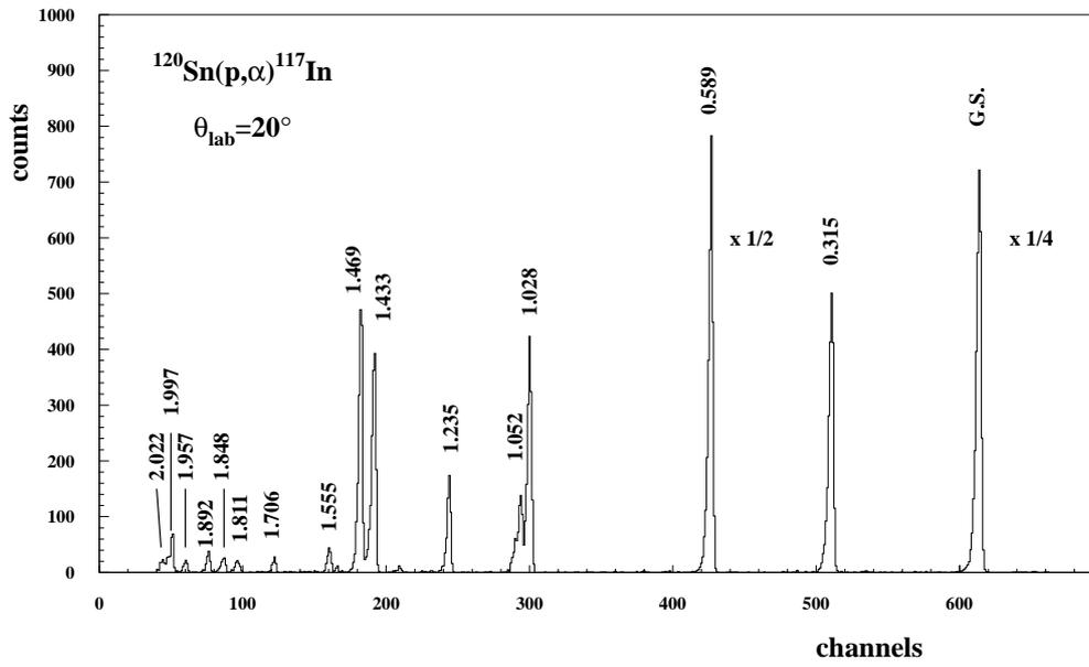
Fig. 1. Energy spectrum of  $\alpha$  particles measured at  $20^\circ$  for the  $^{120}\text{Sn}(p,\alpha)^{117}\text{In}$ .
