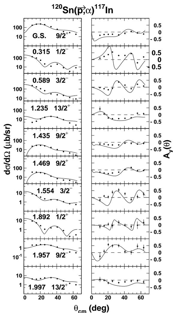
**Fig. 3.** Angular distributions of cross sections and asymmetries for some  $^{117}\text{In}$  states populated in the  $^{120}\text{Sn}(\text{p},\alpha)^{117}\text{In}$  reaction. Dots refer to the experimental values and solid lines to the cluster DWBA calculations.
