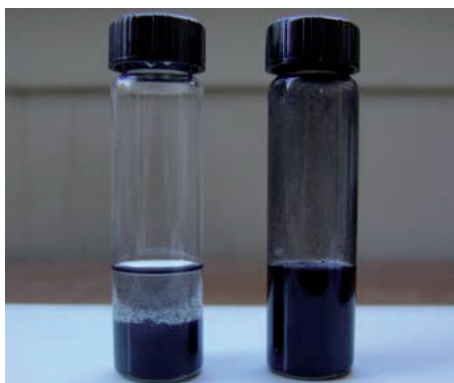
Figure 1. (Left) as supplied MWNTs in a DCPD mixture after one hour and (Right) functionalized MWNT and DCPD mixture after three days
