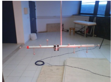
Fig. 4 : Pendulum with the MotionPOD On the photo, we see the different markers and the MotionPOD fixed on the pendulum
