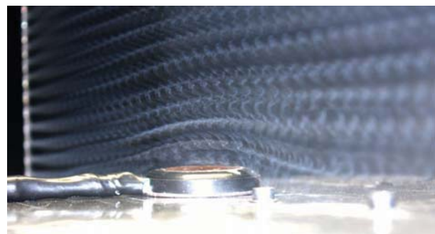
b - Re_L = 67000 , short exposure, flash
