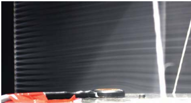
c - Re_L = 67000 , long exposure, no flash, wake region
