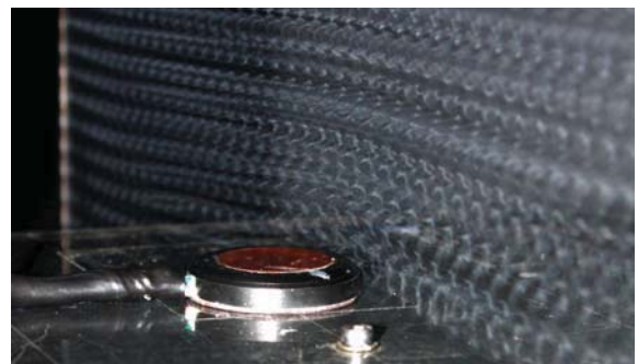
b - Re_L = 56000 , short exposure, flash Off-axis flow near the probe
