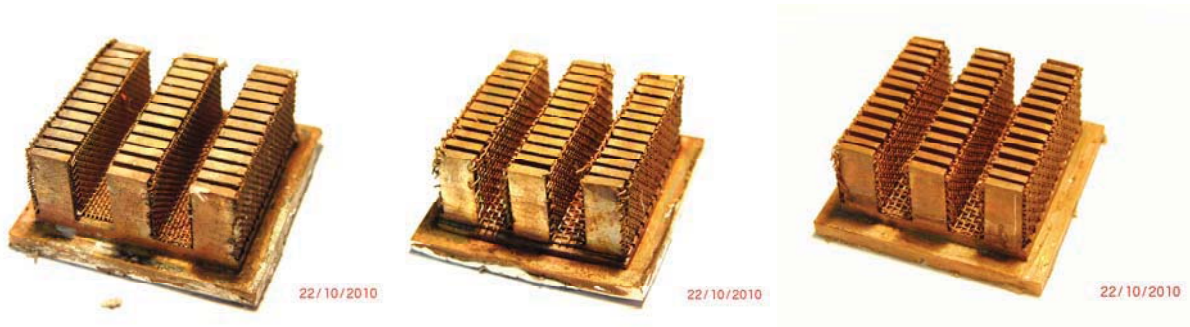
Figure 2. Photograph of NTS samples with wire mesh (N-10-0.6-03, N-10-0.6-0.5, N-10-1.0-0.5) .
