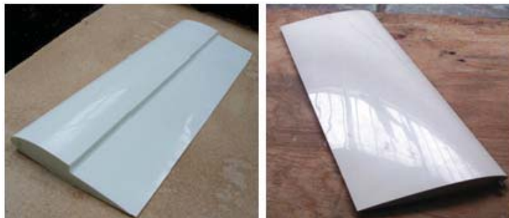
(a) 2415-5 (b) NACA 2415 Fig. 6 a,b. Airfoil models for testing.
