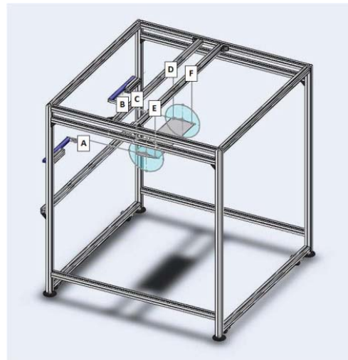
Fig. 1. Structure of the aerodynamic balance.
