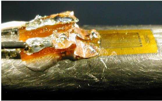
**Fig. 5.** Copper foil soldered to connection tab and the strain gage's tab after failure.
