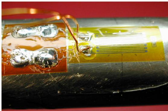
**Fig. 2.** Thin wires soldered to the strain gage's tab.
