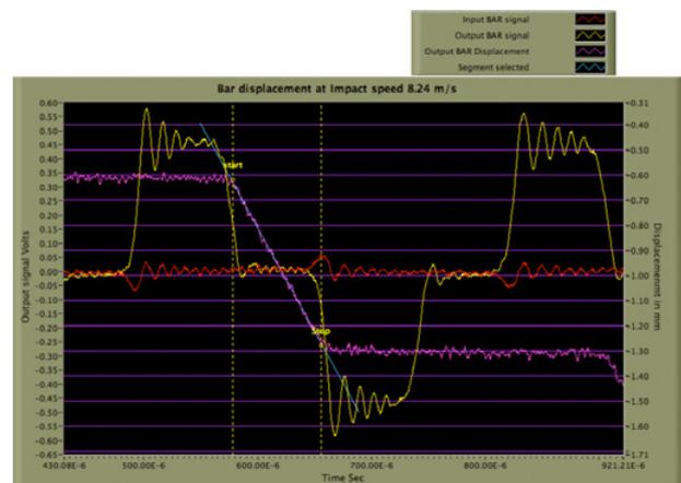
**Fig. 9.** Output bar displacement and wave traveling.
