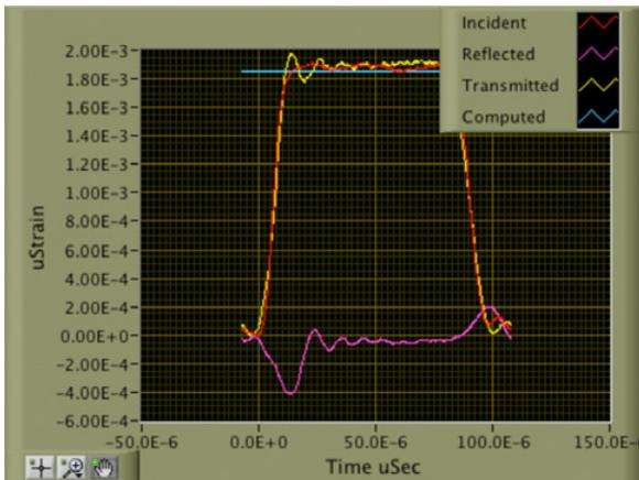
**Fig. 7.** HSR test result of Stress-Proof. Impact velocity of 21.9 m/s.
