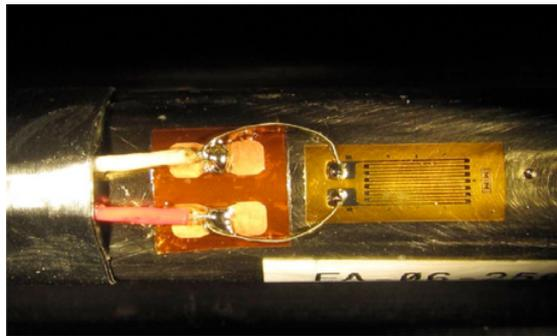
**Fig. 6.** Connection Tab soldering technique.
