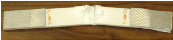
Fig. 6. 0° Tensile specimen broken.
