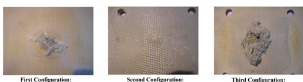
Fig. 12. Detail view of the top surface of the first part (8mm) of the backing.
