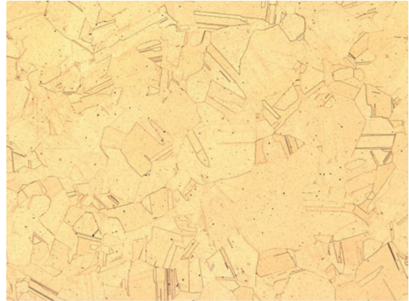
Fig. 3. Example of micrograph of the brass: for low percentage of zinc the two materials are soluble at the solid state and create the single phase FCC_A1.
