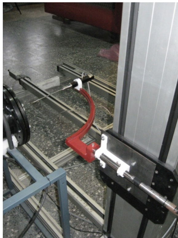
Fig. 3. Probe on the three directional traverse mechanism
