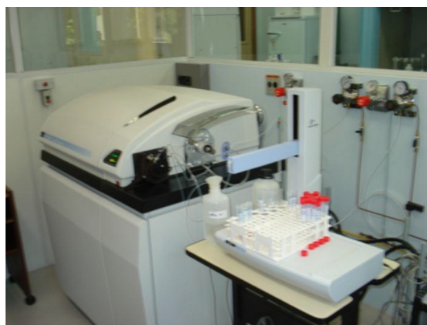
Figure 3. ELAN DRC-2 ICP-QMS and automatic sampler at CDTN.
