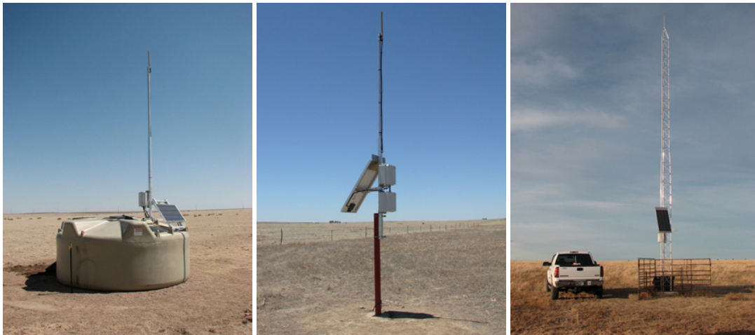
Figure 2. Elements of the RDA: Left: the new 1-PMT surface detector used in Auger South. Middle: the standard communication-only station. Right: the commercial tower used for the concentrator station and selected locations within the array.
