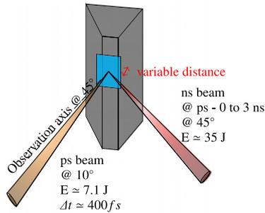
**Figure 3.** Schematic of the target respectively to the laser beams and to the observation axis.
