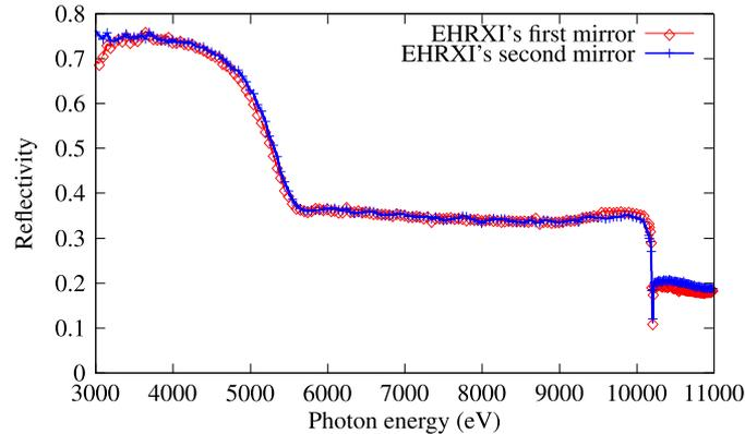
**Figure 1.** EHRXI's mirrors reflectivity vs X-ray energy at 0.6°. Two mirrors were tested: the first mirror of EHRXI (blue crosses) and the second one (red diamonds).
