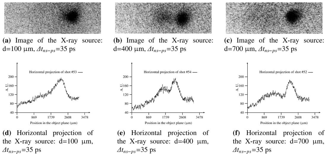
**Figure 4.** Evolution of the X-ray source shape with the distance between the CH foil and the tantalum converter.
