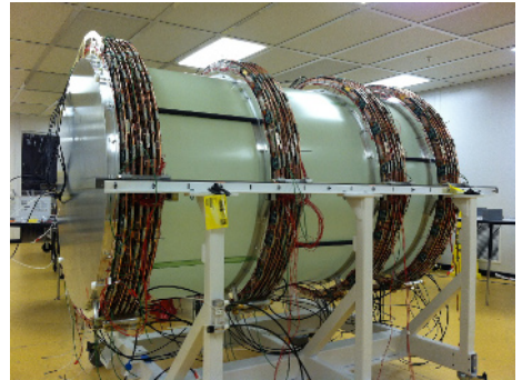
Figure 6. The GlueX Forward Drift Chamber (FDC) assembled and ready for final testing. The FDC consists of four separate packages, each with six chambers. Each chamber provides signals both from the wires and the cathode strips. Both the upstream and downstream cathode planes are instrumented for readout. This provides information on the position along the hit wire improving the pattern recognition.
