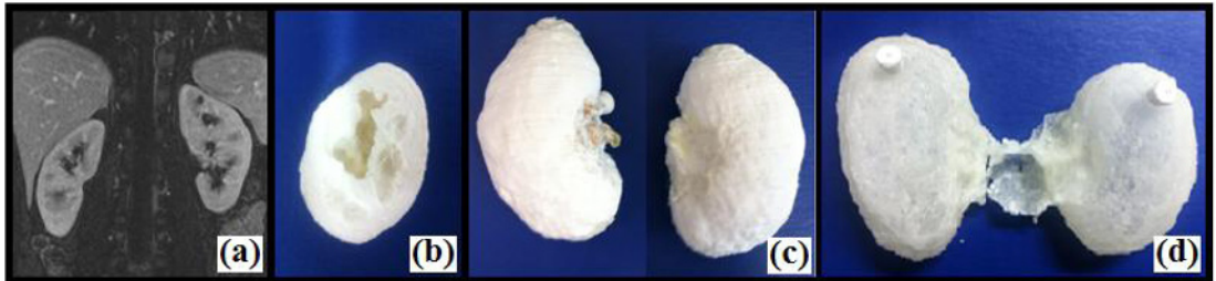
Figure 1. (a) TC used for 3D kidneys reconstruction. (b) Image showing the preservation of internal structures of the ABS renal phantom. (c) External view of the ABS renal phantom. (d) Static renal anthropomorphic phantom prepared with acrylic.
