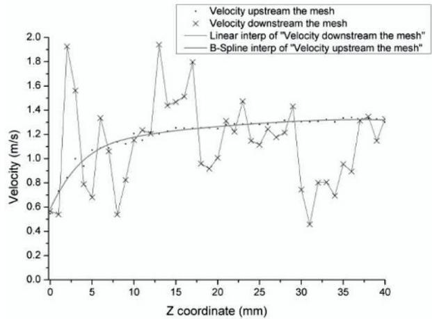
**Figure 5.** A comparison of velocity profile immediately upstream and downstream the wire mesh in a vertical measuring line.
