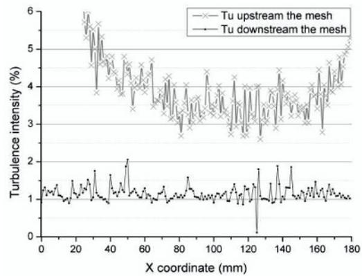
**Figure 6.** A comparison of turbulence intensity profile immediately upstream and downstream the wire mesh in a horizontal measuring line.
