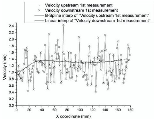
**Figure 4.** A comparison of velocity profile immediately upstream and downstream the wire mesh in a horizontal measuring line.
