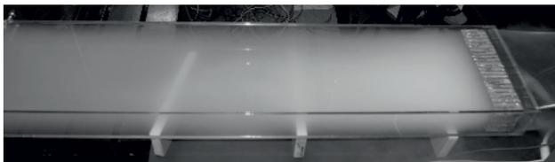
**Figure 2.** Smoke visualization of the flow upstream the mesh.
