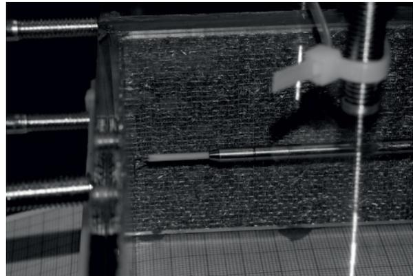
**Figure 3.** Position of the probe during measurement of horizontal line upstream the mesh.
