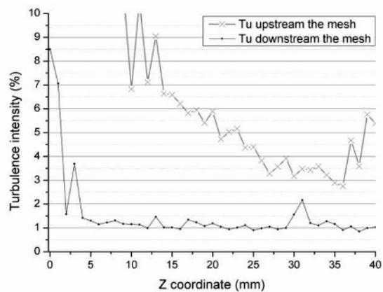
**Figure 7.** A comparison of turbulence intensity profile immediately upstream and downstream the wire mesh in a vertical measuring line.
