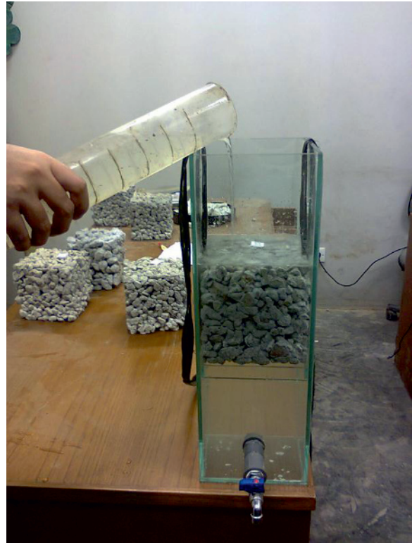
Fig. 6. Water infiltration test
