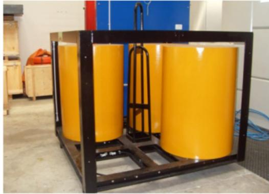
**Figure 1.** Pallet of (mock-up) drums, constructed at INFN-LNS for test purposes.
