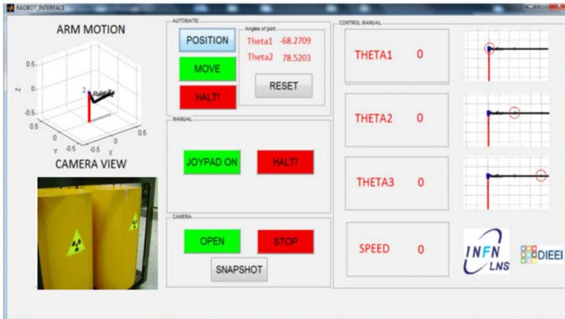
**Figure 9.** RadlBot operator interface.
