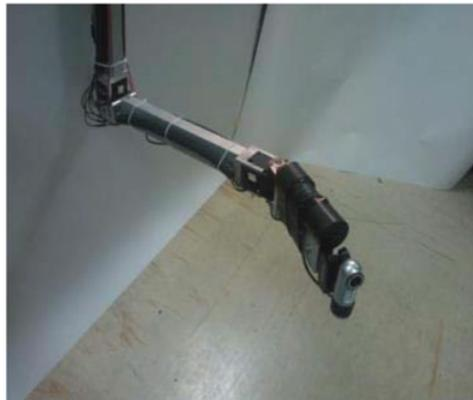
**Figure 8.** RadIBot detail of the last link and end-effector.
