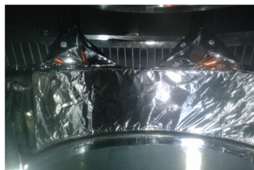
Figure 3. Top: schematic drawing of the OSIRIS secondary spectrometer highlighting in green the neutron paths through the Be filter after scattering by the sample. Bottom: photograph of the actual Be-filter assembly inside the OSIRIS tank, showing the radial arrangement of the Be wedges as described in the main text. The Be blocks are enclosed within a thermal shield and additional multilayer insulation. Two copper legs link the top of the filter assembly to closed-cycled refrigerator (CCR) heads located outside the vacuum tank. In this photograph, the radial collimator can be seen behind the filter.
