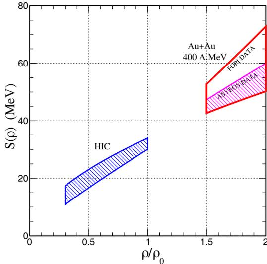
Figure 3: Density dependence of the symmetry energy. The region enclosed by a thick line at high density refers to old Au+Au FOPI data on elliptic flow. The hashed magenta region to new ASYEOS experiment preliminary data. The blue hashed region (HIC) is mainly from Sn+Sn isospin diffusion data (see text).
