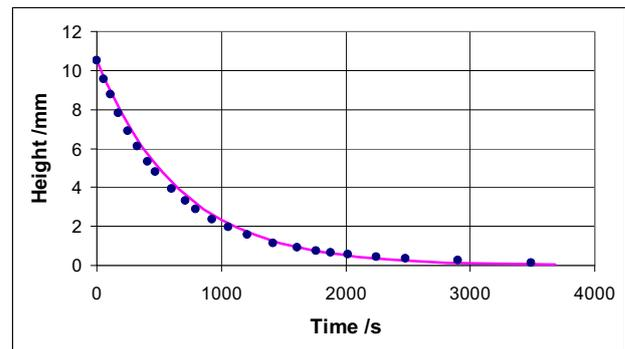
**Figure 6.** Capillary  $d = 0.05$  mm, experimental data (circles) and calculated (line).
