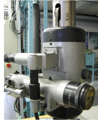
Figure 4. Lomo KM-6 cathetometer.
