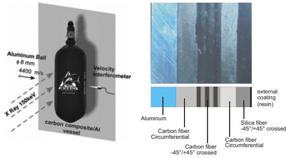
**Figure 1.** Cut view with description of the Aluminum-Composite vessel (left) and comparison of cut-view with model (right).
