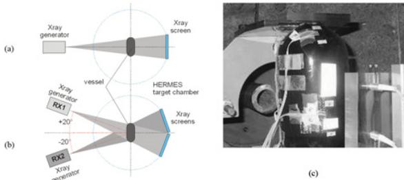
**Figure 2.** Schematic view of Xray configuration: (a) single beam (b) double beam (c) Composite-Aluminum pressure vessel inside the target chamber.
