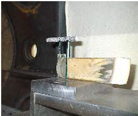
(c) Reverse impact specimen in target chamber
