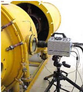
(b) Target chamber and high-speed camera
