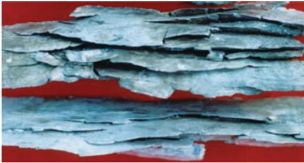
**Figure 3.** The recover samples show shear failure characteristics.
