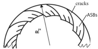
**Figure 5.** Schematic diagram of shear cracks and shear bands spacing.
